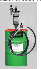
The new Viper Mk II kit includes an upgraded lubricant pump, built specifically for the Viper WRL. Two pump options are available the standard unit delivers 4.5kg/min. while the optional high volume unit delivers 13kg/min for fast lubrication of large diameter ropes, for further reduced down time.
